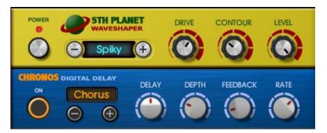
The synth has two fixed *insert effects*, a Waveshaper and a Chorus/Delay. These effects are referred to as insert effects because they are inserted into the signal chain between the synth and the mixer. The master output of the synth is fed through Waveshaper and then through the Chorus/Delay before eventually arriving at the mixer.
