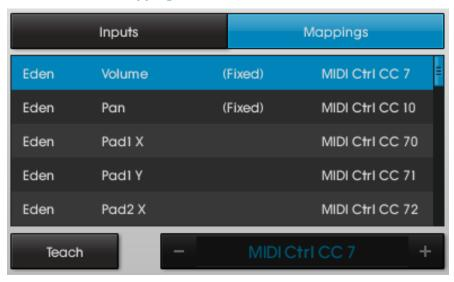
The MIDI Controller Mappings determine which MIDI controllers NanoStudio's instruments will respond to. In the example below, MIDI controller 70 has been set to control the mixer's send 1 volume.
